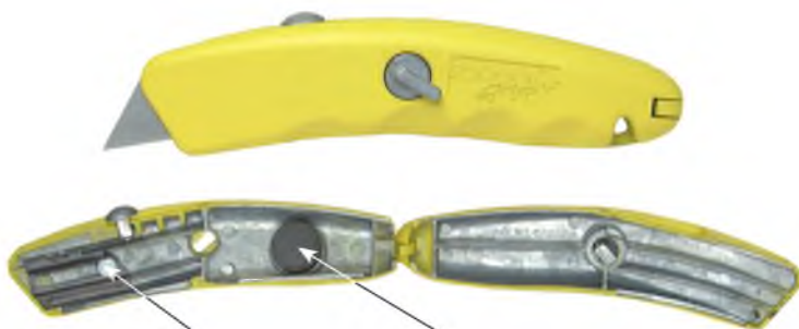
Retractor locked in place. Magnet holds the blades.
